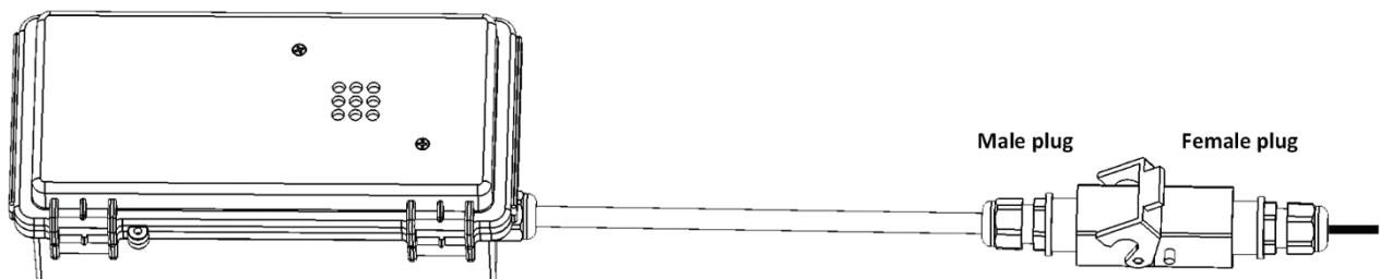
Figure 3: CO<sub>2</sub> Sensor Attached to Connector
