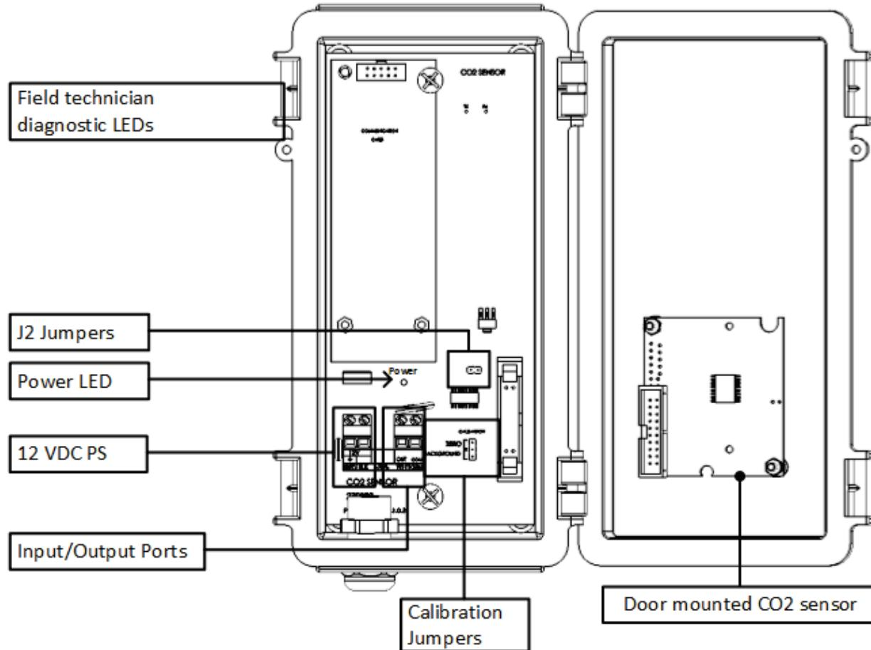
Figure 1: CO<sub>2</sub> Sensor
