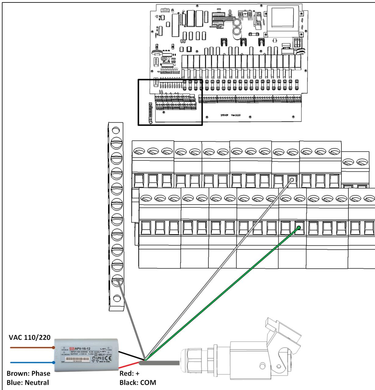
Figure 12: AC-2000 Power Supply Wiring
