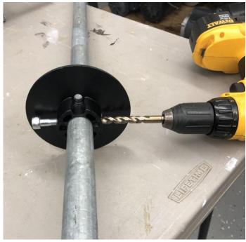
The drum bolts have an 8 mm Allen head and are inserted on the opposite side of the belt attachment when it is unwound.
