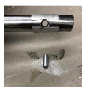
The inside of the pipe needs to have the rough edges and points filed off with a rat-tail file before installing it onto the shaft. Make a 3/8-inch dowel 1 inch long from a 3/8 bolt to hold the sleeve in place while sliding the pipe over it. Use a little WD40 inside the pipe so it slips more easily over the sleeve.
