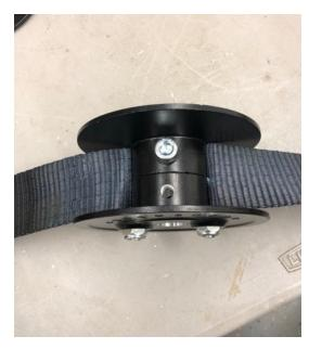
Place pipe brackets on both sides of the belt drum, and as needed between the drums to carry the pipe without it sagging.
