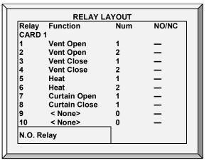
If you have installed Current Sense relays, the controller defines them automatically. Current sense relays transmit to the user's PC the amount of the current being passed to the relay and send alarms when the current is too low or too high. In addition, you can view the daily electricity consumption in History. Refer to Current Sense Relay Calibration, page 116 for calibration instructions.
