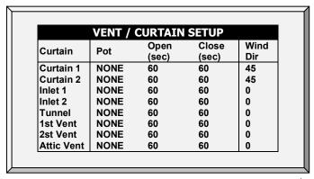
Set full open/full close time (in seconds) for Curtains, Tunnel, 1<sup>st</sup> & 2<sup>nd</sup> Vent, and Attic Vent.
