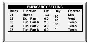
• **Relay:** The Controller determines the relay numbers automatically from the position in the controller in which the Emergency Switch card is installed.
