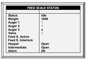
This screen shows the status of different areas of the feeding apparatus. illustrates the system components.
