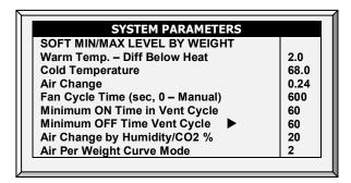
Warm Temperature - Difference Below Heat: Differential below the heat temperature (refer
