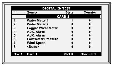
A '1' implies a shorted input, a '0' an open input. The digital sensors operate with dry contact inputs such as the Arad Water Meter, or micro-switches.
