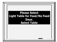
1. Select Feed and press **Enter**. The Light parameters screen appears. These parameters configure the Light functions on feed days.
