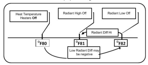
Figure 2: Radiant Heater Differentials
