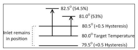
Figure 27: Example of Inlet Opening Hysteresis
