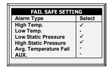
The Platinum Pro/Rotem Pro has six options besides controller failure or power off to activate the fail-safe relay. Apply the additional settings by using the '+/-' key:
