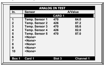
The readings can vary from 0 to 1023. The values displayed in the 'Value' column indicate that the analog sensor is operating or not according to the following:
