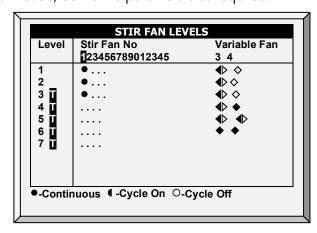
In the Stir Fan Level table set the speed in percentage that you want the variable speed fan to work at (by levels). For each level, program the stir fans' cycle. Configure the actual speed in Analog Output, page 124.
