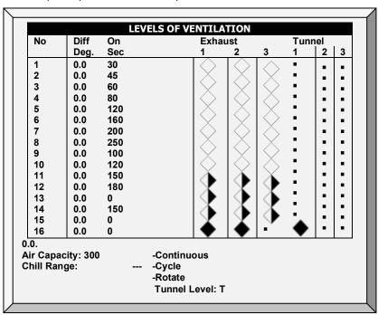
NOTE The number appearing under Exhaust and Tunnel is refers to the numbers defined in Installation.
