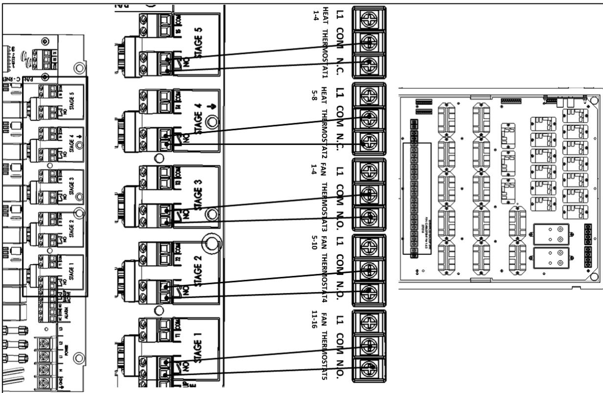
Figure 7: Wiring Between RDT-5 and FBU-27 SE
