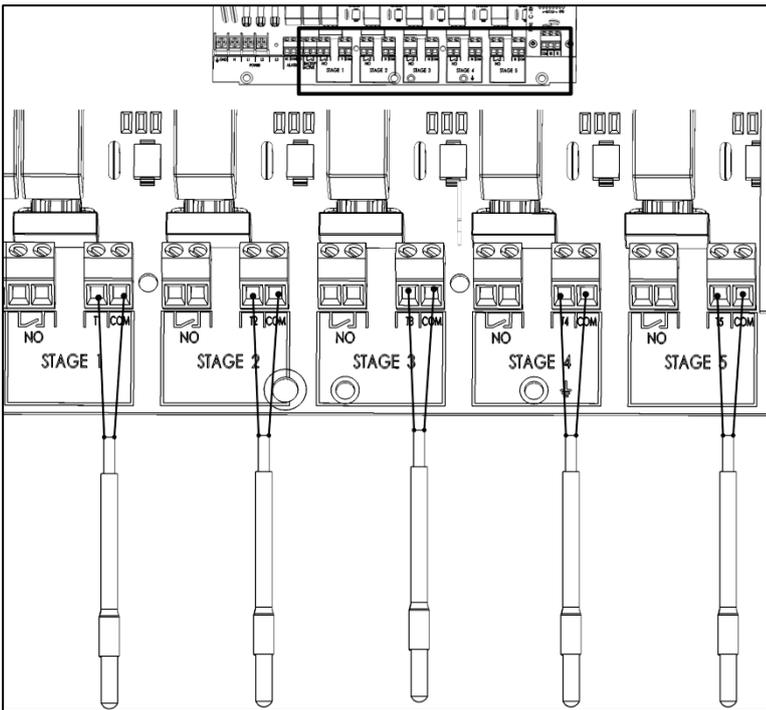
Figure 8: Wiring Between RDT-5 and FTS-2
