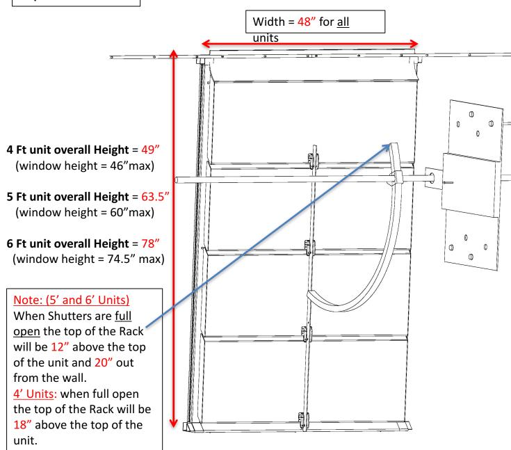
Note: 8 inches needed above Shutter unit if installing Shaft Hangers.
