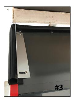
\* If installing on frame openings <u>smaller</u> than specified in Step 2, it may be necessary to trim the Air Baffles to meet your specific requirements.
